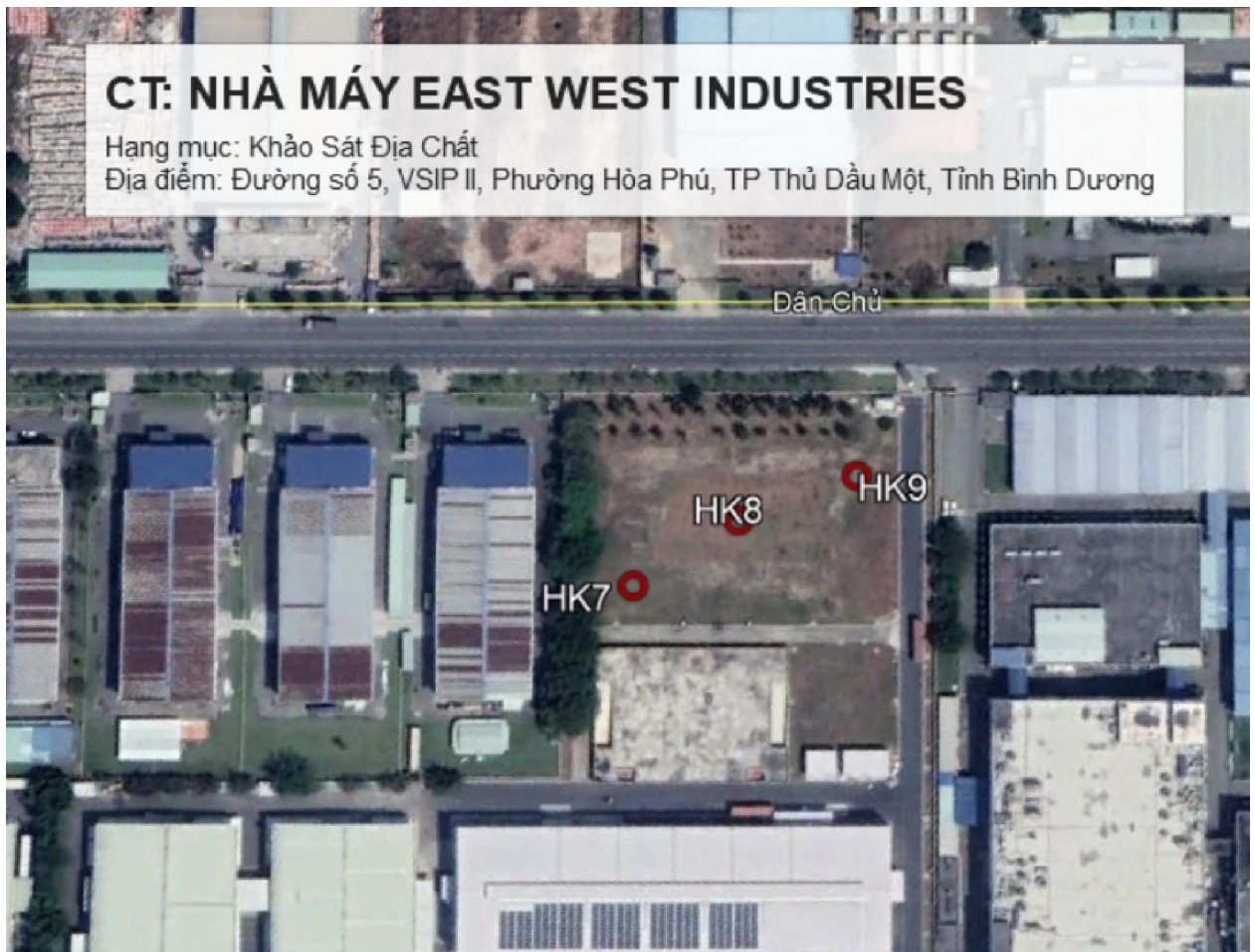
Figure 1: Layout of Borehole Locations
