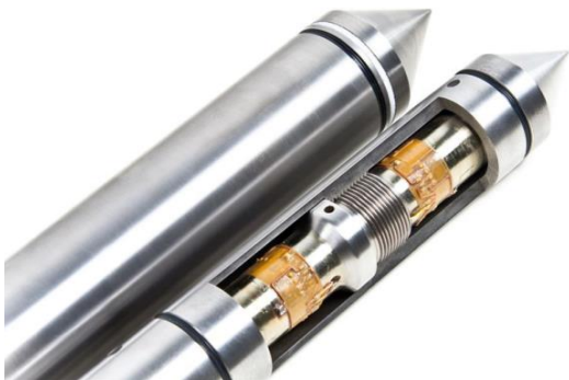
Picture 4: The electronic cone AC10CFIIP type and Data acquisition system: GME500 IP65 type
