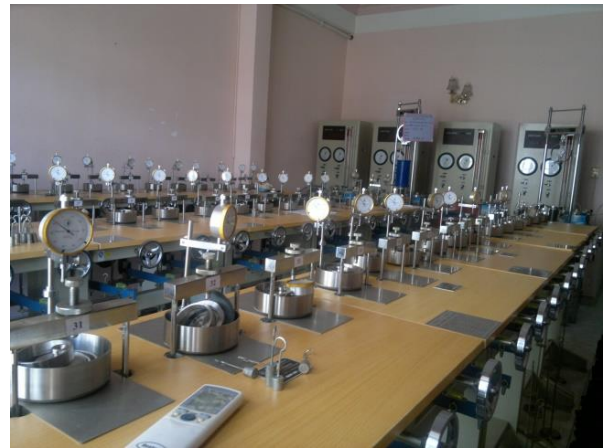
(Picture 10: Consolidation test)
