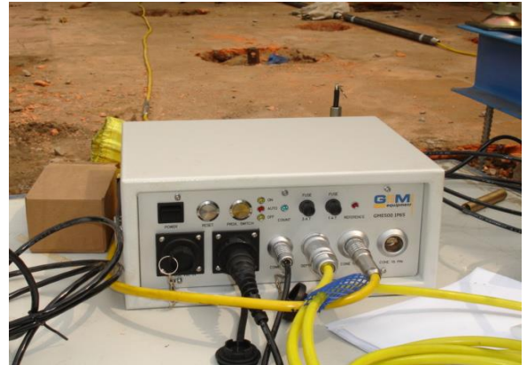
Picture 4: The electronic cone AC10CFIIP type and Data acquisition system: GME500 IP65 type
