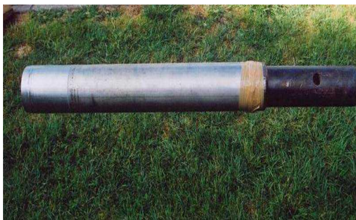
(Picture 2: The typical thin-walled tube)
